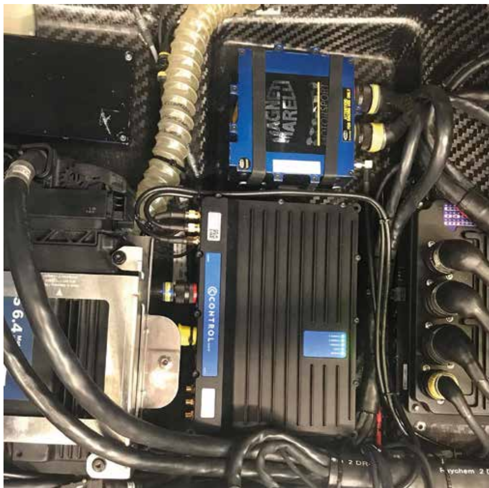
The Control TLM-P1 Modem installed in a modern racecar alongside a logging unit, ECU and power distribution modules
